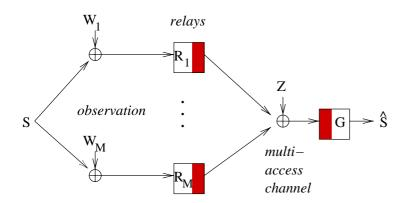
*Scenario:* M sensors observe an information source and relay their readings over a broadcast channel to the destination.
